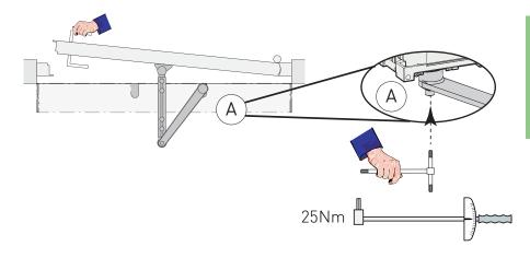
NB: open the door slightly and tighten the screw of the arm support seat [A] at 25 Nm (as shown in the figure). If a torque wrench is not available, use a
