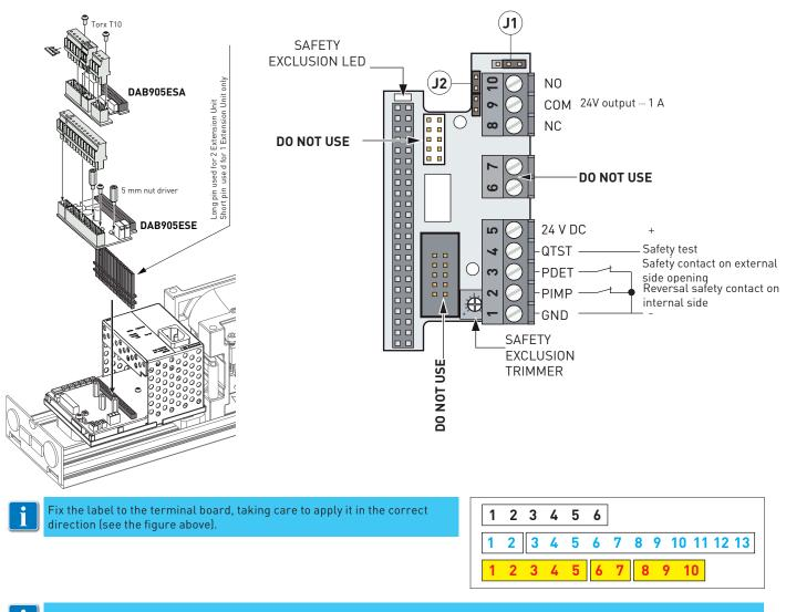
Remove the jumpers if a safety sensor is connected to terminals 1-2 and 1-3.
