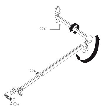
• In the case of automations with left-hand opening, you must invert the assembly of the articulated arm as shown in the figure.
