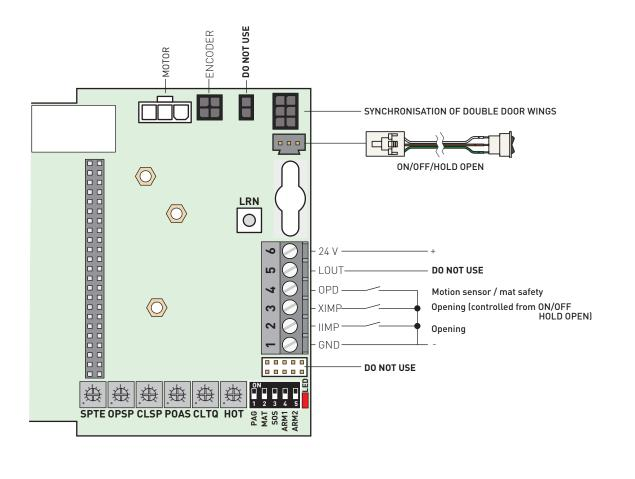
Fix the label to the terminal board, taking care to apply it in the correct direction (see the figure above).
