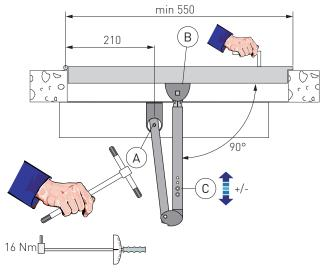
NB: open the door slightly and tighten the screw of the arm support seat [A] at 16 Nm (as shown in the figure). If a torque wrench is not available, use a hexagon wrench of the type shown in the figure, gripping it on the long side and tightening very firmly.
