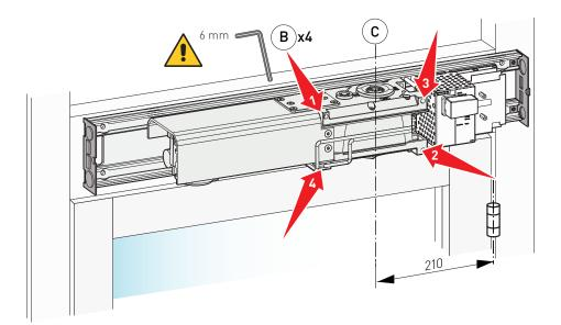
• Fix the motor by tightening the screws [B] supplied, in the sequence shown in the figure.
