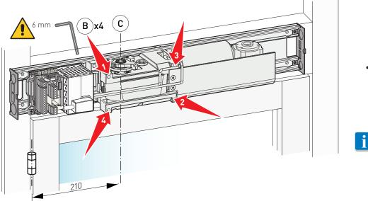
• Fix the motor by tightening the screws [B] supplied, in the sequence shown in the figure.
