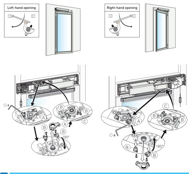
The following operations must be carried out with the arm installed and the door closed.
