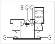
Fix the door wing to the carriage with screws [a]. The outer wheel of the carriage must not protrude beyond the dimension of the door wing.
