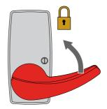
In the event of maintenance, malfunctioning or emergency, lower the lock release lever LOKSBM (if installed) and move the door wings manually into the open position.
