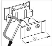
The measurements of the code 0KP369 floor guide for glass door wings are indicated in the diagram.
